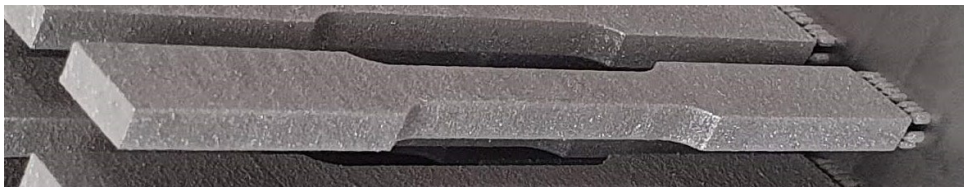
Figure 3.3: As-built coupon still attached to the print bed with supports visible.
