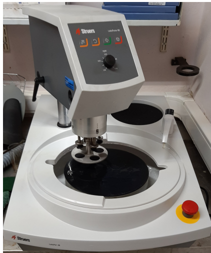
Figure 3.5: The Struers LaboPol-30 used to polish the samples.
