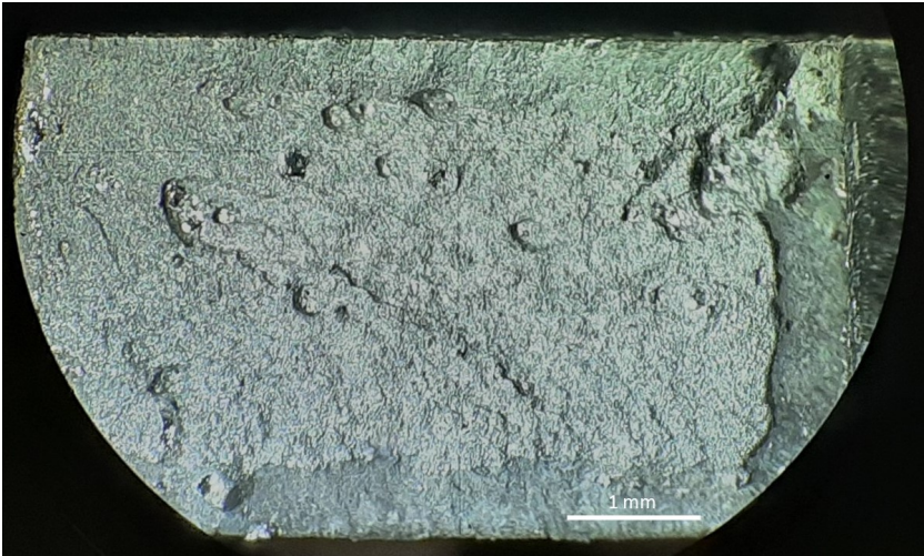
Figure 4.1: Fracture surface of coupon P5.
