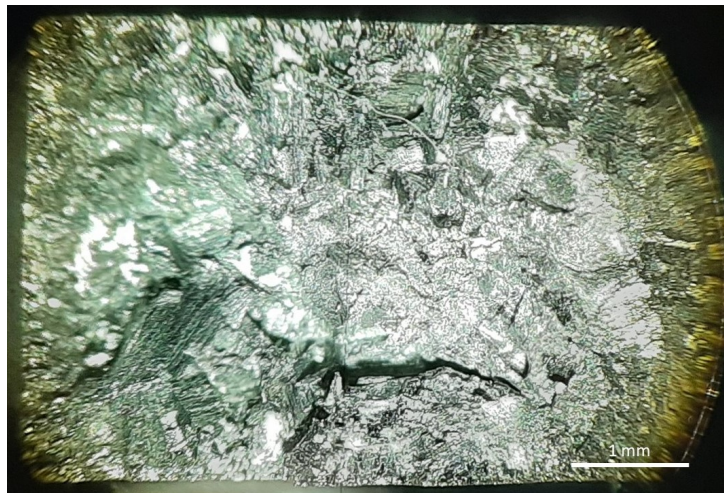
Figure 4.6: Fracture surface of a coupon treated at 1100°C.
